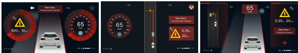
Figure 3.11 State 2 TOR Designs (Design A, Design B, Design C - left to right)
