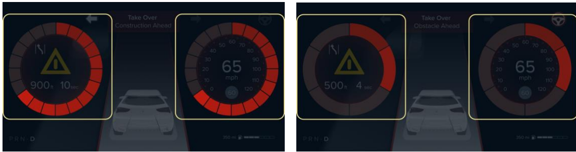
Figure 4.4 Highlighting countdown element in Design A during LU TOR (left) and HU TOR (right)
